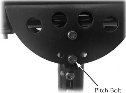
6) Not commonly necessary but the actual forearm platform can be adjusted forward or backward. First remove padded cover that is held on by Velcro. Then loosen platform bolts. Slide platform into desired position and reinstall bolts. Finally, reattach padded cover.
